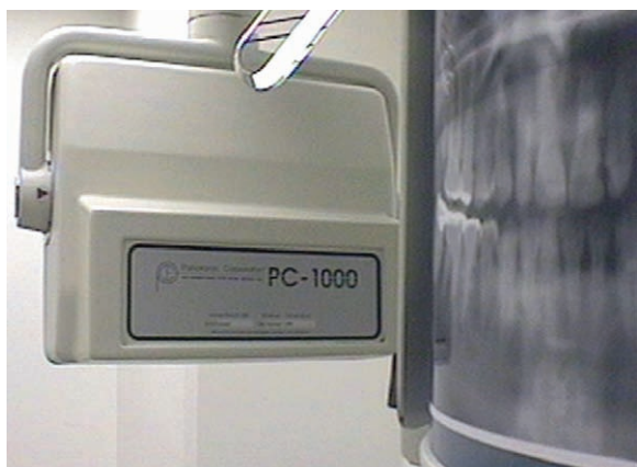
Fig. 1.6 The panoramic latent image is created as the film cassette moves past the secondary slit. The production of the latent image is simulated using the print of a panoramic radiograph
