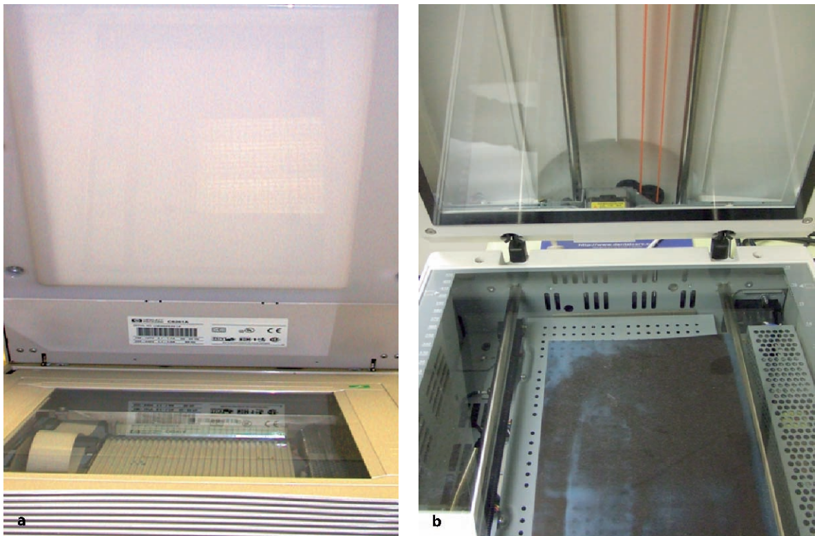
Fig. 3.1 a Nikon CoolPix scanner with transparency adaptor in lid sufficient for extraoral radiograph duplication. b Panoramic radiograph placed for digitization in an alternative flat bed scanner, the Epson FinePix Z2 with transparency adaptor
